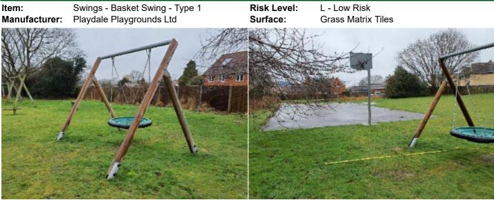
**Finding:** The overhanging branches forms a hard object within the falling space of the equipment in contravention of the requirements of BS EN 1176 Part 1
