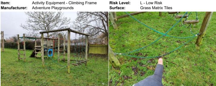
Finding: The rope is making contact with the surface
