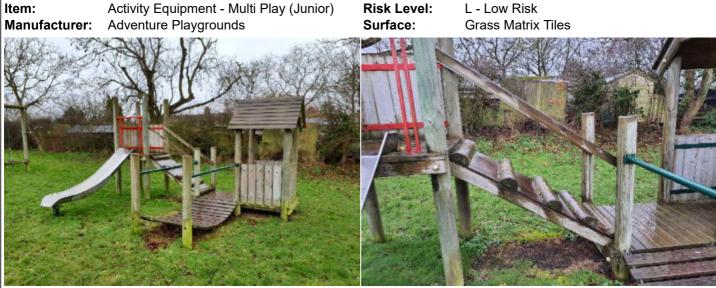
**Finding:** The unit is easily accessible and should have the **Action:** Monitor - No remedial work recommended appropriate barriers installed to meet the requirements of BS EN 1176 Part 1 as the height of the unit exceeds 600mm
